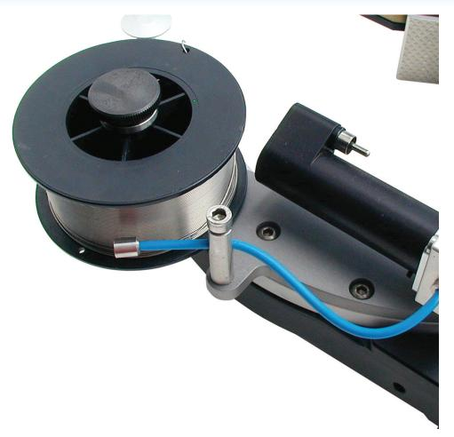
A range of open weldheads for NB pipe c/w options of wire feed, oscillation, AVC. A further range of tube to tube sheet heads to suit boiler applications.
